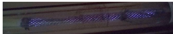
Figure 7 Filamentary discharges homogeneously distributed in the air gaps at the braid / cable insulation interface.
