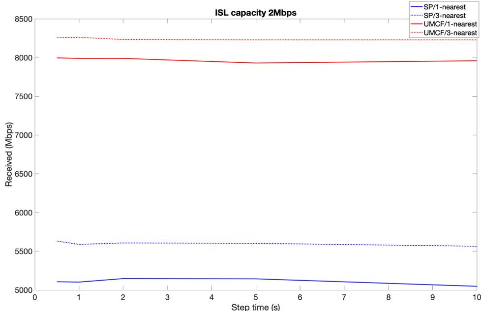
Figure 3: Impact of the time step between consecutive routing tables generations on the performance of proposed routing algorithms (11919.67 Mbps of data are sent during this experiment).
