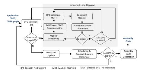
${\bf Fig.\,4.}\ {\bf Proposed\ compilation\ flow\ supporting\ standalone\ execution\ of\ nested\ loops\ and\ modulo\ scheduling\ of\ innermost\ loop$
