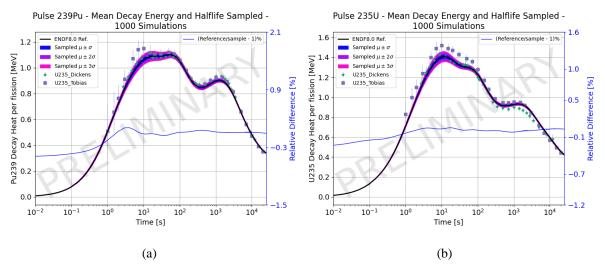
Figure 3: Total decay heat per fission as a function of cooling time. (a) <sup>239</sup>Pu fission pulses with ENDF/B-VIII.0 decay data library and (b) <sup>235</sup>U fission pulses with ENDF/B-VIII.0 decay data library.
