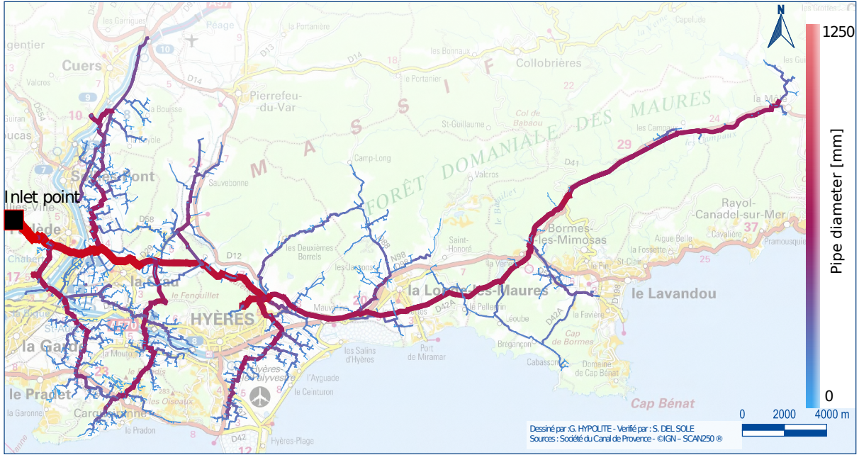
Figure 1: Map of the A network, colors and lines thickness representing the pipe diameter
