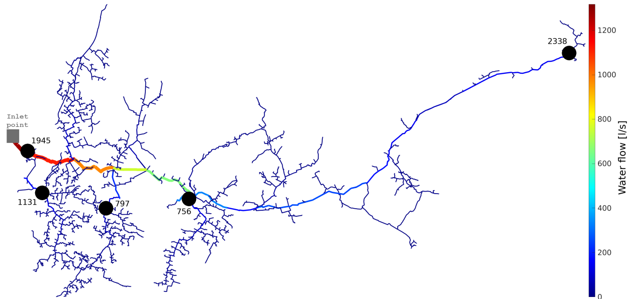
Figure 8: Water flow in network A on June 30 and distribution of hydraulic potential (black circles; the associated values are in MWh/year).
