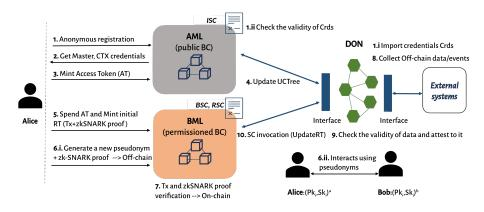
Fig. 1: Overview of DARS Framework, comprising an Access Management Ledger (AML), a Business Management Ledger (BML), and a Decentralized Oracle Network (DON).
