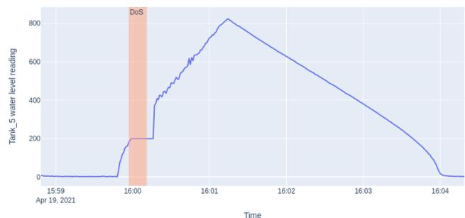
Fig. 1. Effect of a DoS attack on a tank water level reading from HITL testbed
