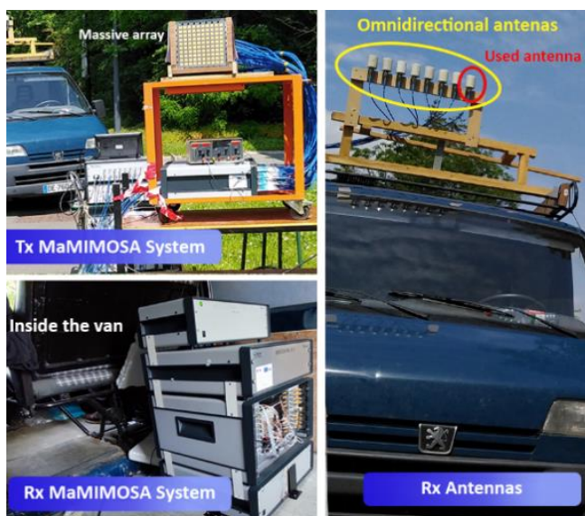
Figure 2. Tx-Rx antenna systems.
