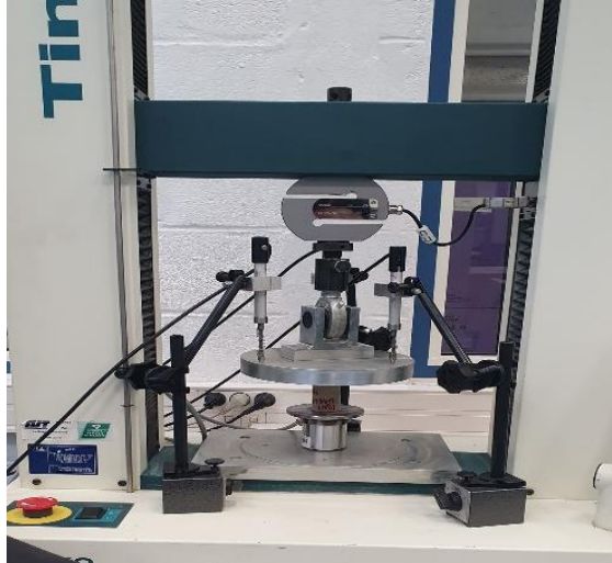
Fig. 1. Compression test of geopolymer materials
