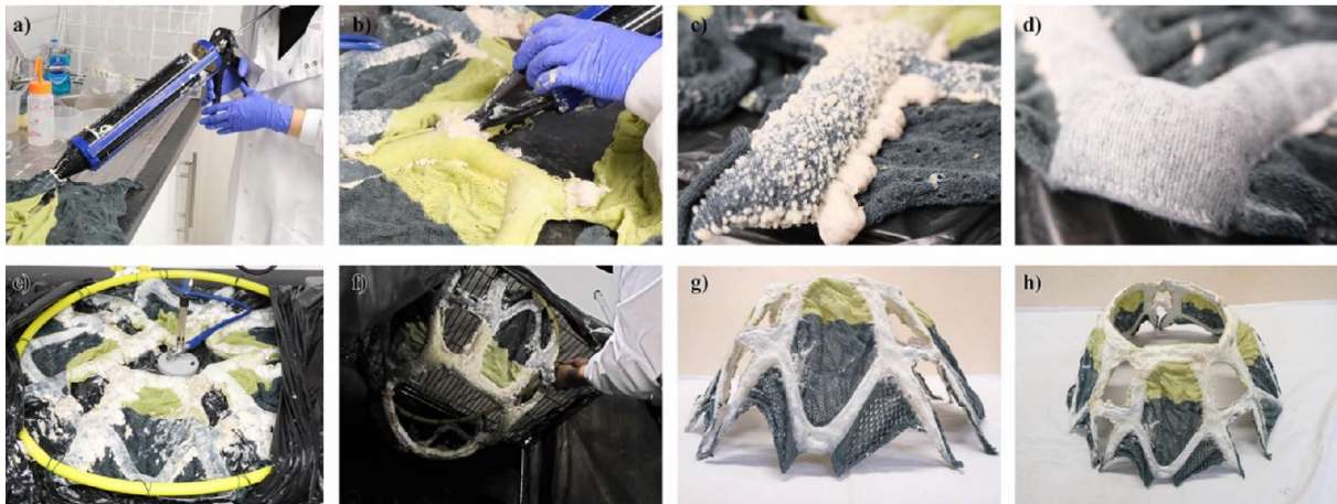
Figure 4. Paste extrusion gun (a), filling tubular components (b), filled fabric tube (c), during the mycelium process (d), assembly of the soft pre-grown textile structure into the upside-down hanging construction (e/f), air dried dome from different perspectives (g/h) (Scott et al., 2022)
