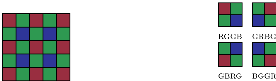
(a) The Bayer CFA, by far the most commonly used CFA. (b) The four potential patterns that arise from the Bayer CFA.
