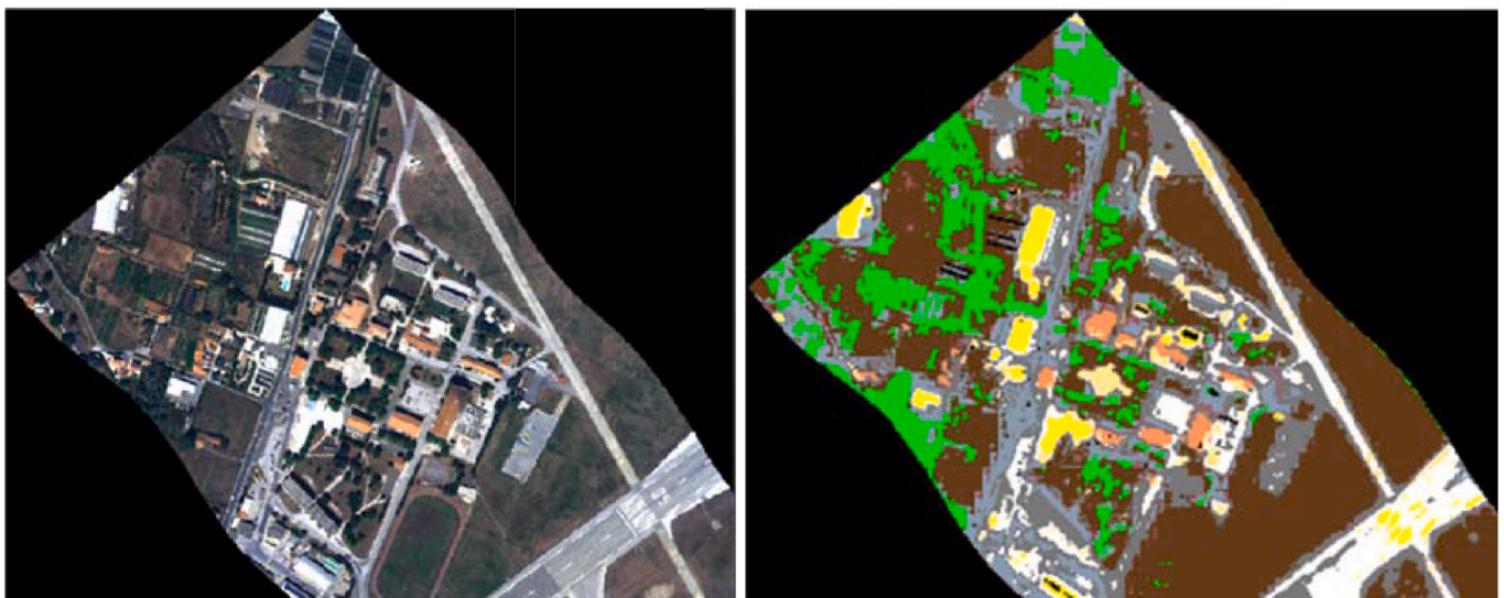
Fig. 15 Left: RGB reference image of Toulon at 2.5 m GSD. Right: Classification map with (#1,T,O).
