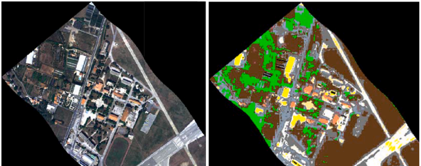
Fig. 15 Left: RGB reference image of Toulon at 2.5 m GSD. Right: Classification map with (#1,T,O).
