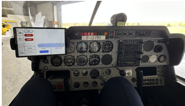
Fig. 1. Tablet interface placed close to the cockpit.
