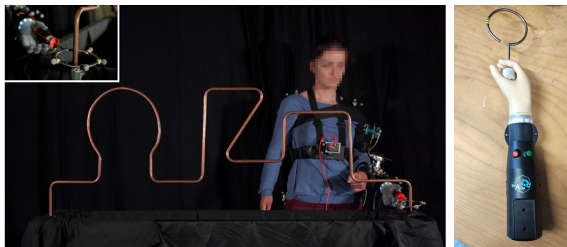
Fig. 5. Left: Experimental setup: Cybathlon wire-loop task with the adapted prosthetic device. The upper left insert shows the handle hold by the prosthetic hand. Right: View of the forearm prosthesis used for demonstration with asymptomatic users
