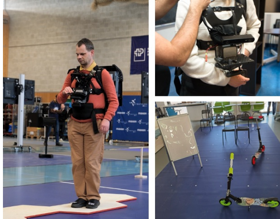
Fig. 6. Left: View of our pilot using the A-Eye device at the Cybathlon-Challenges event in Zurich. Top Right: Close-up view of the system featuring a 3d stereoscopic camera above and a 2-degree-of-freedom kinesthetic feedback device below. Bottom Right: View of the “Sidewalk” challenge, the aim of which is to advance to the finish line without touching obstacles on the sidewalk.
