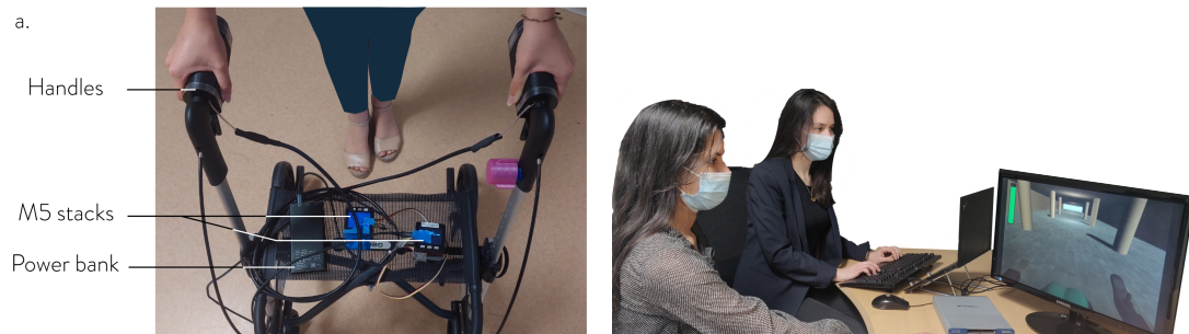
(a) Experimental setup : The photo shows the handles mounted on the walker. Signals are amplified and sent to the handles by the M5 Stacks controllers connected via WiFi. The motors are powered through the M5 Stacks cabled to a power bank.
