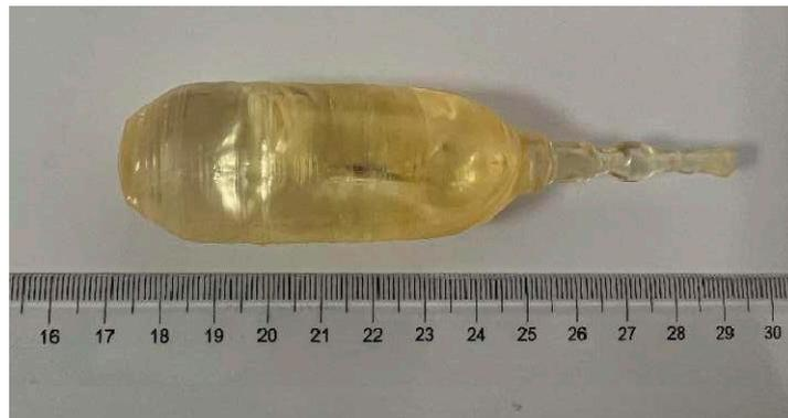
**Figure 1.** Photograph of as-grown 5 at.% Yb:CALYGLO crystal.
