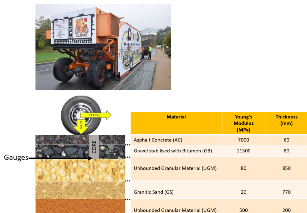
Figure 11. MLS10 testing system and pavement structure.
