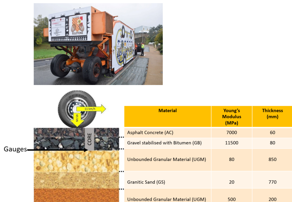
Figure 11. MLS10 testing system and pavement structure.
