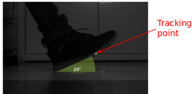
Figure 8. The position of the participant foot at the downward movement starting time.
