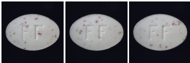
Fig. 2. Example of variability of textures in the good pill class of the MvTech dataset [8]. Though the structure of the pills is the same (ellipsoids with big Fs engraved), the red spots are spread randomly and might be confused with anomalies.
