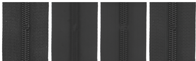
Fig. 4. Three sorts of normalization from rigid to flexible. From left to right: image without normalization, image after normalization using all whole images, using whole nearest images, finally using nearest patches.
