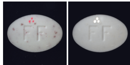
Fig. 3. Effect of normalization (left: before, right: after) on the pill class of the MvTech dataset [8]. The normalization removes all ”normal” red marks while keeping the anomalies.
