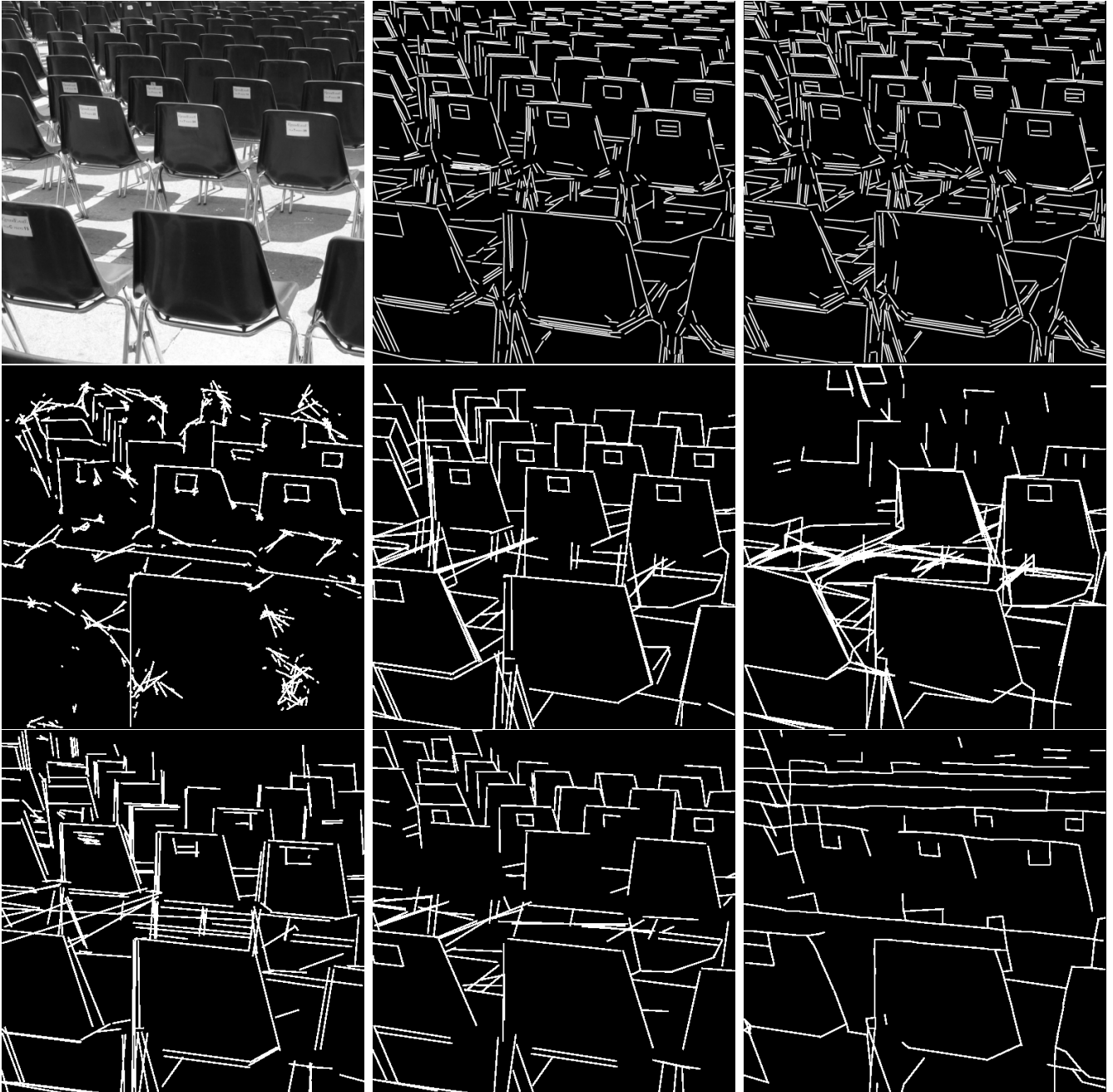
Figure 10: Comparison of eight line segment detectors on an “out of domain” image, a photograph of chairs: original image “chairs” results of LSD (2008), EDlines (2011), AFM (2019), TP-LSD (2020), ULSD (2021), LETR (2021), M-LSD (2021), SOLD2 (2021). The first two detectors are handcrafted and based on edge growing followed by an a contrario detection threshold. The last six are obtained by sophisticated, mainly supervised, deep learning methods.
