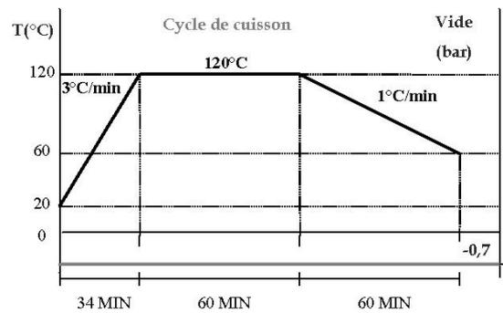
Figure 3: Cycle de cuisson / *Cure cycle*
