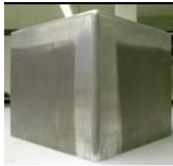
Figure 1. Tool used for the manufacture of the corner fitting
