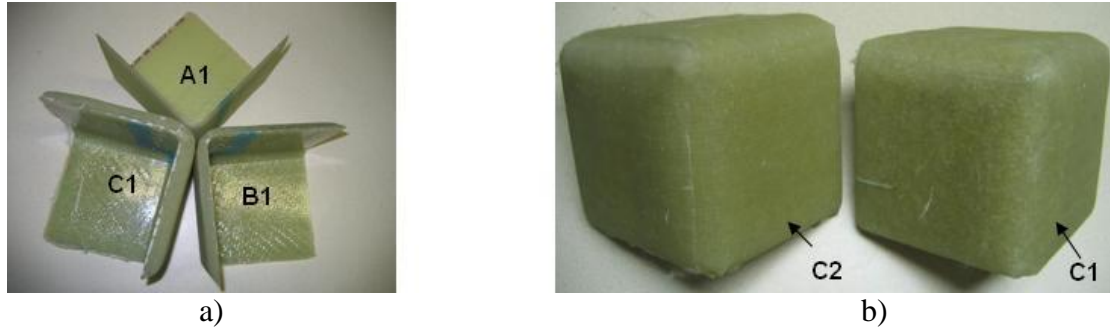
Figure 7. a) Corner fittings A1, B1 and C1 laid-up with respectively 3, 9 and 15 plies using "short cycle" b) Corner fittings made of 15 plies cured resp. with the long (C2) and the short cycle (C1).
