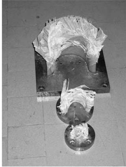
Figure 10. Comparison of rupture modes at different scales.
