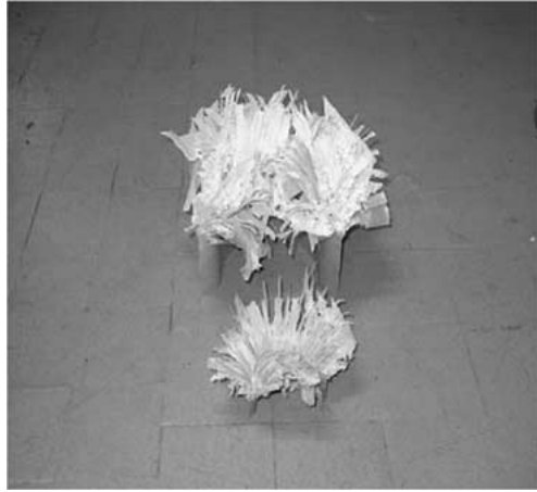
Figure 11. Presentation of the different rupture modes in statics.
