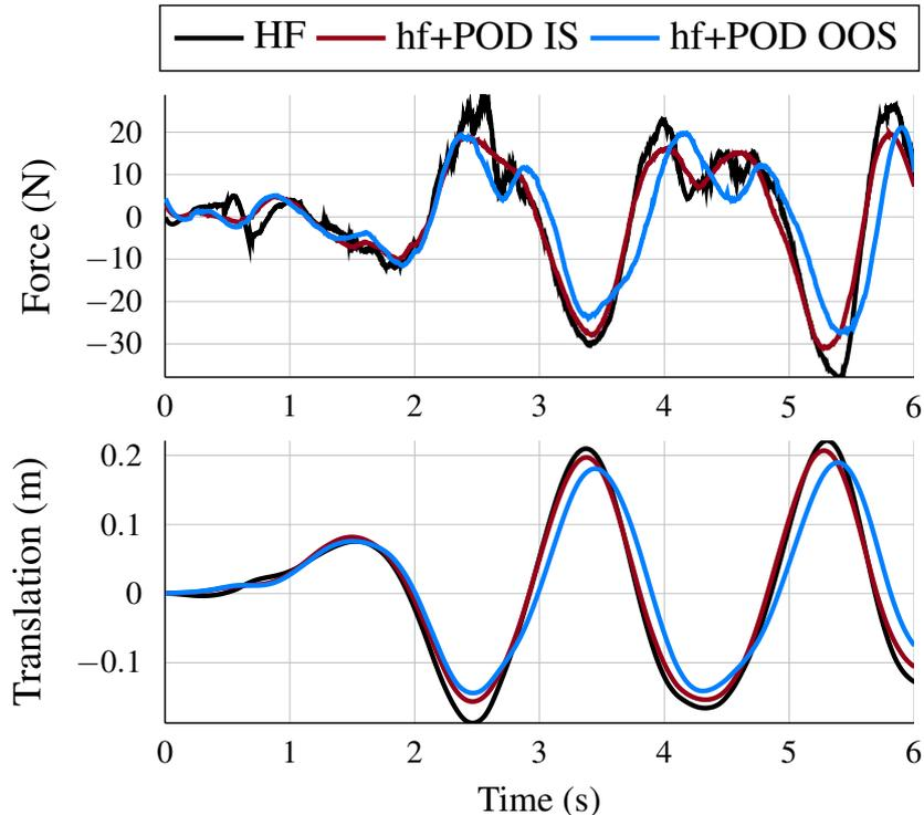
Figure 12: Evolution of the force acting on the body and the heave motion of the body.
