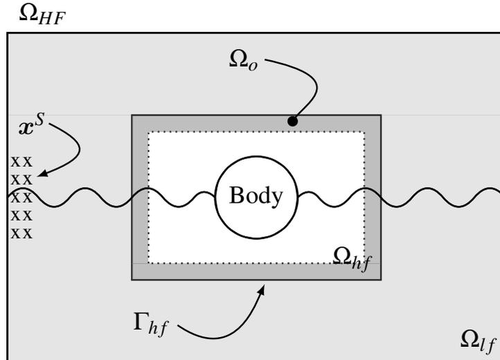
Figure 3: Domain decomposition for the coupling methodology. The overlapping domain  $\Omega_o$  is dark-gray colored. The high-fidelity domain  $\Omega_{hf}$  is the union of the white and dark gray domains, and the low-fidelity domain  $\Omega_{lf}$  is the union of the light and dark gray domains.
