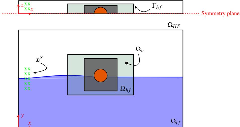
Figure 11: Domain decomposition for the sphere simulation.
