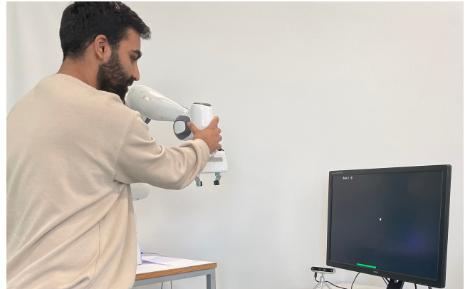
Figure 1: A user playing the Pong game by physically interacting with the robot while a depth camera is used to detect his skeleton (S2).
