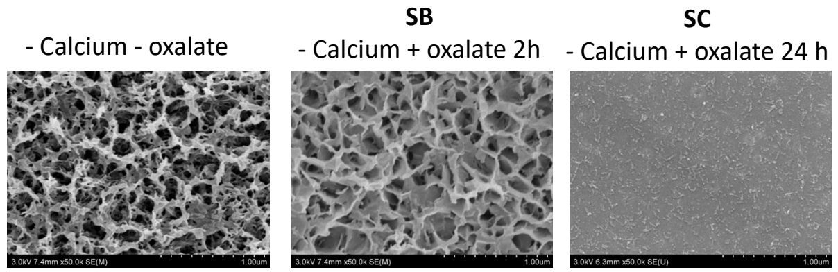
Fig. S4: SEM-FEG images of the initial CHA substrate and at the end of the experiment for SB and SC
