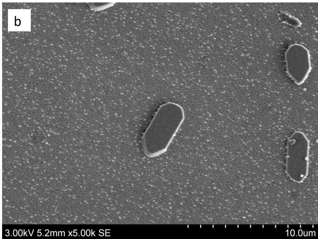
Fig. S6: a,b) Crystallization of CaOx at the outlet of the microchannel after infusion of oxalate solutions on CHA for 24h (SC)
