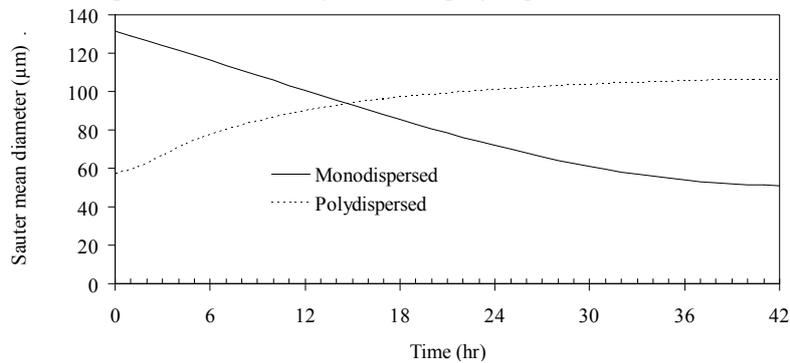
Figure 4. Predicted variation of Sauter mean diameter for monodispersed and polydispersed size distributions
