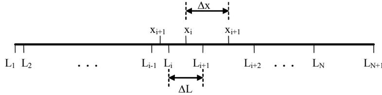
Figure 1. Convention for discretization of the particle size domain
