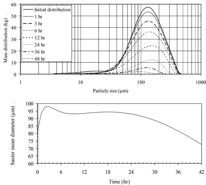
Figure 6. Simulation of particle size distribution (top) and Sauter mean diameter (bottom) variation with the PBM
