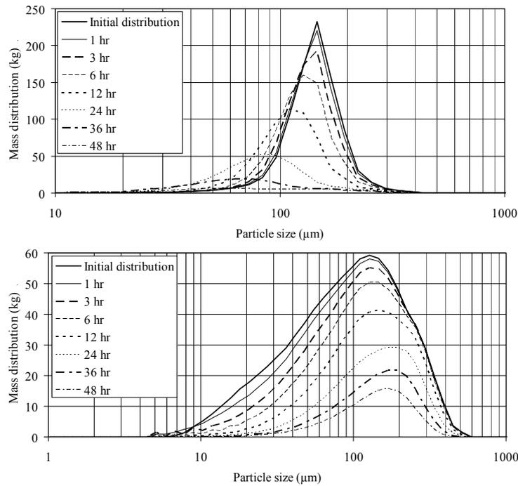
Figure 2. Results from Equation (5) with monodispersed (top) and polydispersed (bottom) particle size distributions
