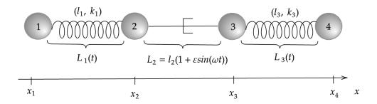
Figure 3: Four-sphere swimmer where the middle arm connecting spheres 2 and 3 is the activated part. Springs have rest lengths  $l_i$  and spring constants  $k_i$ . Distances between the spheres are given by  $L_1(t)$ ,  $L_2(t)$  and  $L_3(t)$ . In this case, the motion of the middle arm is prescribed as:  $L_2 = l_2(1 + \varepsilon \sin(\omega t))$ .
