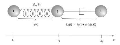
Figure 1: Three-sphere swimmer as proposed by Montino and DeSimone in [13]. Two spheres are connected by a spring with rest length  $l_1$  and spring constant k. The third sphere is connected by an actuated arm. The distances between the spheres are given by  $L_1(t)$  and  $L_2(t)$ .
