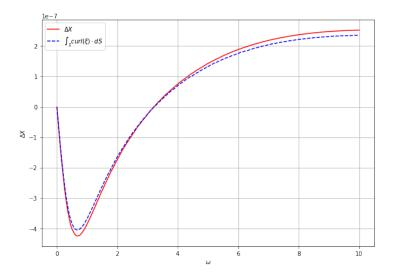
Figure 5: Average displacement per period ( $\Delta X$ , in m) of the swimmer computed directly by integration (in red) and using the circulation of the first-order approximation (13) of curl( $\xi$ ) (in blue), plotted as a function of  $\omega$  (in rad  $s^{-1}$ ), for  $\varepsilon = 0.3$ .
