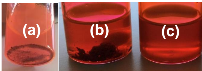
Figure S2. Solubility of EY in 1g of PEGDA resin. (a) PEGDA 250 , BAPO (0.4 wt%), BBOT (0.16 wt%), EY (2 wt%), (b) PEGDA 700 , EtOH (2 wt%), BAPO (0.4 wt%), BBOT (0.16 wt%), EY (4 wt%), (c) PEGDA 700 , EtOH (10 wt%), BAPO (0.4 wt%), BBOT (0.16 wt%), EY (4 wt%)
