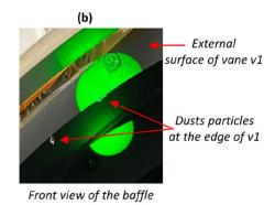
**Figure 4.** (a) Image taken with a conventional camera, positioned at the typical SPAD location, highlighting air scattering, direct edge scattering, and two-stage processes on the vanes. (b) Detection of dust particles on the edge of vane v1.
