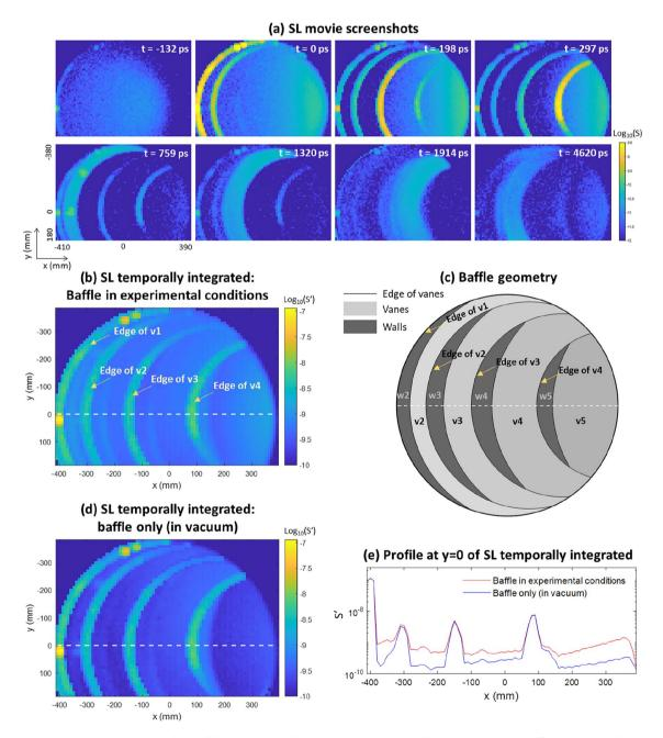
**Figure 2.** (a) Screenshots of the SL movie. (b) Temporal integration of the SL movie. (c) Baffle geometry. (d) Temporal integration of the SL movie, excluding the contributions from OGSE SL and air scattering. (e) Profiles along y = 0 of the SL movie temporally integrated.
