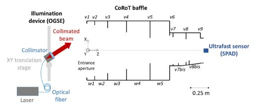
**Figure 1.** Sketch of the experimental setup.
