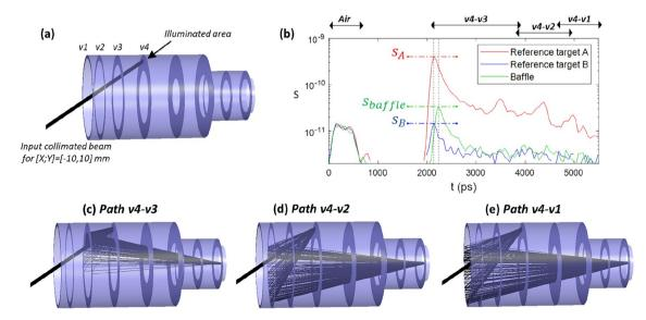
**Figure 5.** (a) Ray tracing depiction of v4 illumination. (b) SL measurement upon vane v4 illumination, with and without a reference target. The ratio  $s_{\text{baffle}}/s_A$  or  $s_{\text{baffle}}/s_B$  enables the deduction of  $R_{\text{baffle}}$  (c-e) Ray tracing illustrations of the different SL paths.
