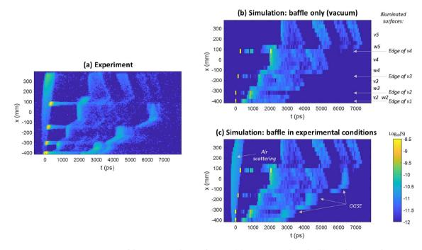
**Figure 3.** Cross-section of the SL movie along x, for y=0. (a) Experimental result. (b) Simulation result with baffle only. Arrows indicate the illuminated element for a given x value. (c) Simulation in experimental conditions, including air and OGSE scattering.
