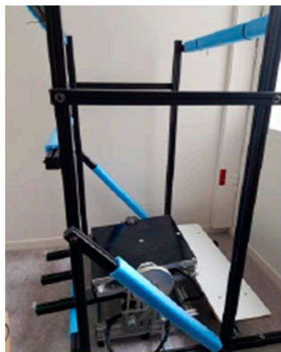
Figure 1. The force platform used in the experimental setup, surrounded by its foam-clad aluminum frame. This platform could be tilted in the AP axis or held stationary horizontally.
