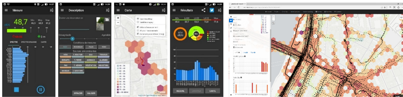
Figure 2: Screenshot of the NoiseCapture application (left) and website for mapping the collected data (right). Source: Bocher et al. [32].
