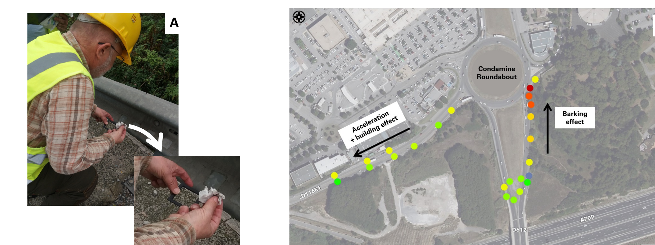
Figure 9 : Different pollution patterns (B) obtained from wiping of the guardrails (A), West of Montpellier city, France.
