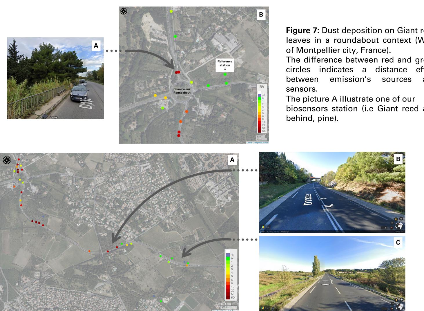
Figure 8: A - Effect of environmental openness on PM concentration on pine needles, D123E2 road sector (West of Montpellier city, France). Red to yellow circles illustrate a mixing effect between closed area and traffic conditions (B). Yellow to green circles mostly illustrate a good pollutant atmospheric dispersion due to an open environment (C).
