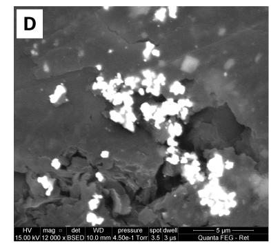
Figure 5 : Observed particulate matters (Scanning Electron Microscopy, SEM). A – Cracked cuticle with multiple micro particles (*Arundo donax* leaf), a potential resuspension source. B – Silica spherule and soot carbon. C – Tire rubber and road wear micro particles aggregated on mycelium matrix. D – Aggregate of metalloid and metal fine dust. E – Copper and iron particle. All identifications have been based on spectral analysis.
