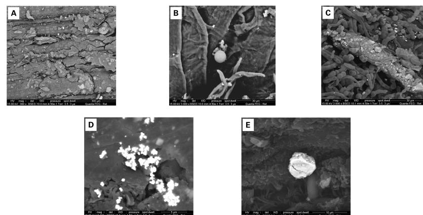
Figure 5 : Observed particulate matters (Scanning Electron Microscopy, SEM). A - Cracked cuticle with multiple micro particles (*Arundo donax* leaf), a potential resuspension source. B - Silica spherule and soot carbon. C - Tire rubber and road wear micro particles aggregated on mycelium matrix. D - Aggregate of metalloid and metal fine dust. E - Copper and iron particle. All identifications have been based on spectral analysis.
