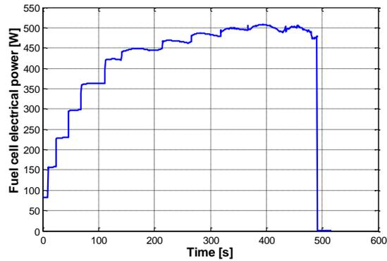
Fig. 2c. Evolution of the FC stack power
