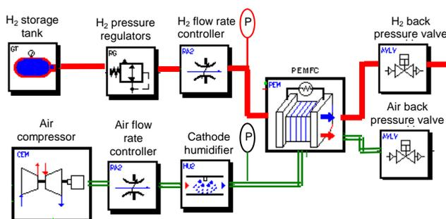
Fig. 1. Simplified scheme of the fuel cell testbench
