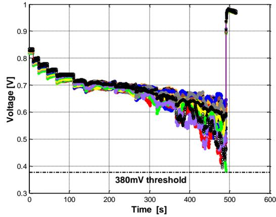
Fig. 2b. Evolution of the 20 cell voltages
