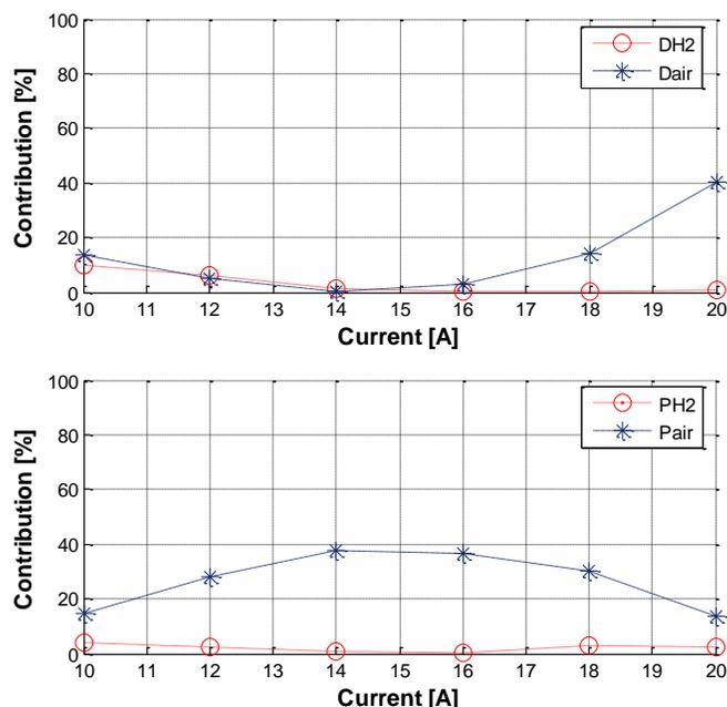
Fig. 5. Contribution of the four studied parameters to the FC voltage
