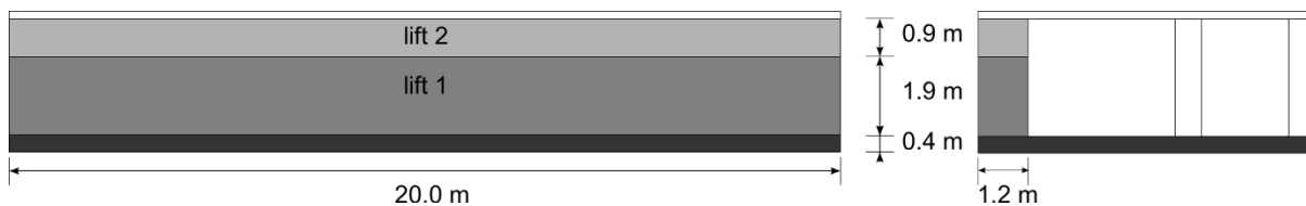
1001 1002 Figure A.1. Geometry of the Civaux mock-up wall: (a) longitudinal view; (b) cross-section.
