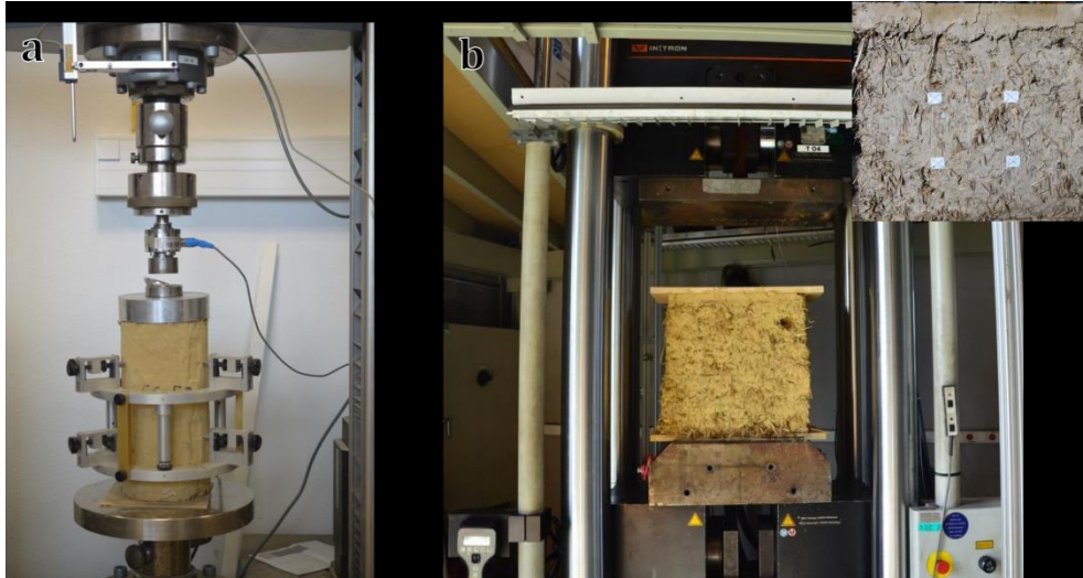
Figure 2. Mechanical tests of cylindrical cob specimens (a) and cob walls (b). 3 loading cycles were applied to the specimens and strain was measured in the central third of the specimen using an extensometer composed of 3 displacement sensors (a) or an optical extensometer for two couples of two targets located in the central third of the wall elements (b).
