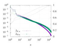
FIG. 3. POD spectra (solid lines, left axis) and cumulative spectra (dotted lines, right axis) for PODs optimized with respect to total kinetic and thermal energy ( $\lambda_{E,n}$ ) and total viscous and thermal dissipation ( $\lambda_{D,n}$ ). The spectra are normalized such that  $\sum_n \lambda_{E/D,n} = 1$ . Power laws fitted to the spectra in the interval  $10 \le n \le 10^3$  are shown for the energy (black dashed line) and dissipation spectra (black dotted line)
