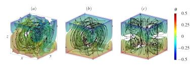
FIG. 2. The snapshot m=1 (a), the conditional mean field given  $L_x < 0, L_y > 0$  (b), and the full mean field (c), shown as isosurfaces of scaled convective heat flux corresponding to  $\Phi_{\rm iso} = 0.05 \cdot {\rm max}_{\Omega}(w\theta)$  and colored by temperature  $\theta$ . In this and the similar plots in Figures 5 and 6 the origin is located in the lower left corner of the cell, and the axes are labeled as shown in (a).
