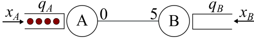
Figure 19. An example of payment queues q_A and q_B in Spider routers (adapted from [90]). Red circles represent unit payments. When the payment arrival rate at A , x_A , is greater than the arrival rate at B , x_B , A eventually runs out of funds, and its payment queue q_A starts to grow. If payments stay in the queue for too long, A will send a message to the payment senders as a warning to reduce their payment rates.
