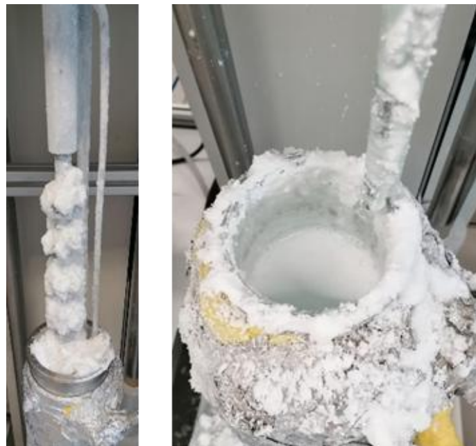
Figure 11. Coagulation in the reactor at a stirring speed of 550 rpm Setup S2+D.
