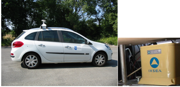
Figure 6. VERT: our experimental vehicle providing ground truth and its on-board IXSEA inertial measurement unit
