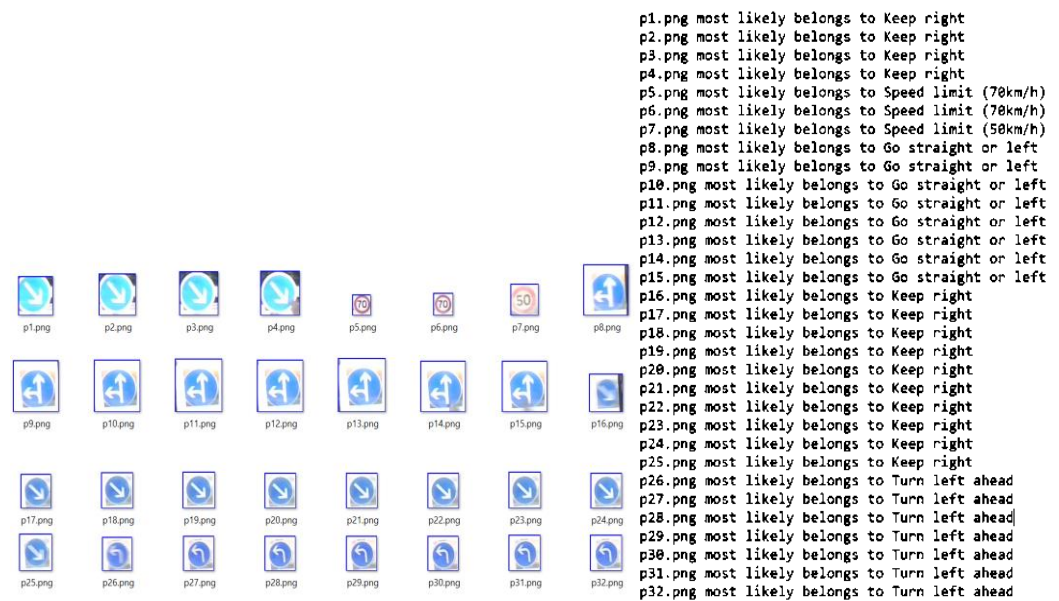
Figure 15. Examples of road sign recognition detected from the webcam of the PC using the TSC-MA.
