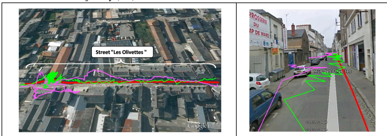
Figure 5: Illustration of the positioning error in the section of street Les Olivettes
