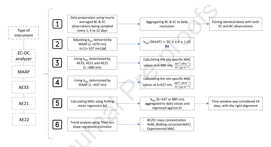
Figure 2. The overall scheme by which to process corrected and normalized eBC mass concentrations in order to obtain site-specific MAC values. More details are provided in sections 2.4, 2.5 and 2.6. (a): 637 nm is the reference wavelength of the MAAP to derive MAAP- equivalent absorption coefficient; (b): 1.05 is the correction factor to the true wavelength (637 nm); (c) Efficient Rolling/ Windowed Operations using "zoo" and "RcppRoll" R packages.
